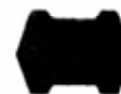
Double "V" ... for serpentine type of drive. BB section only. (uses BB4 fastener)
